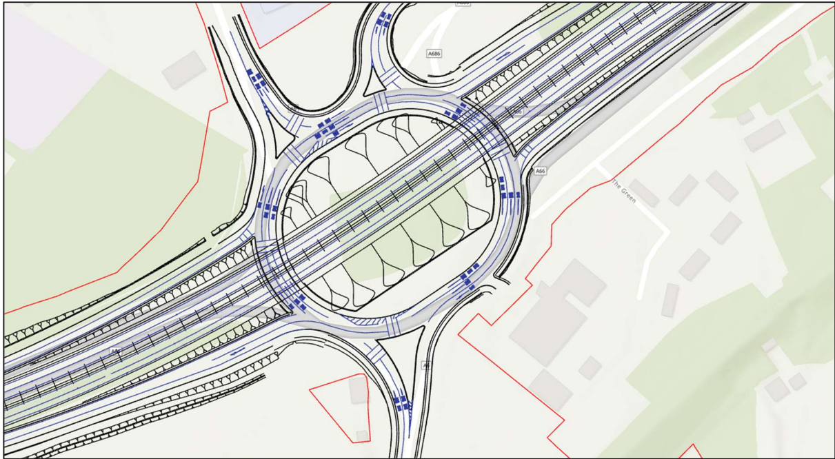
Figure 8-30: A6 / A66 Kemplay Bank Scheme Design
