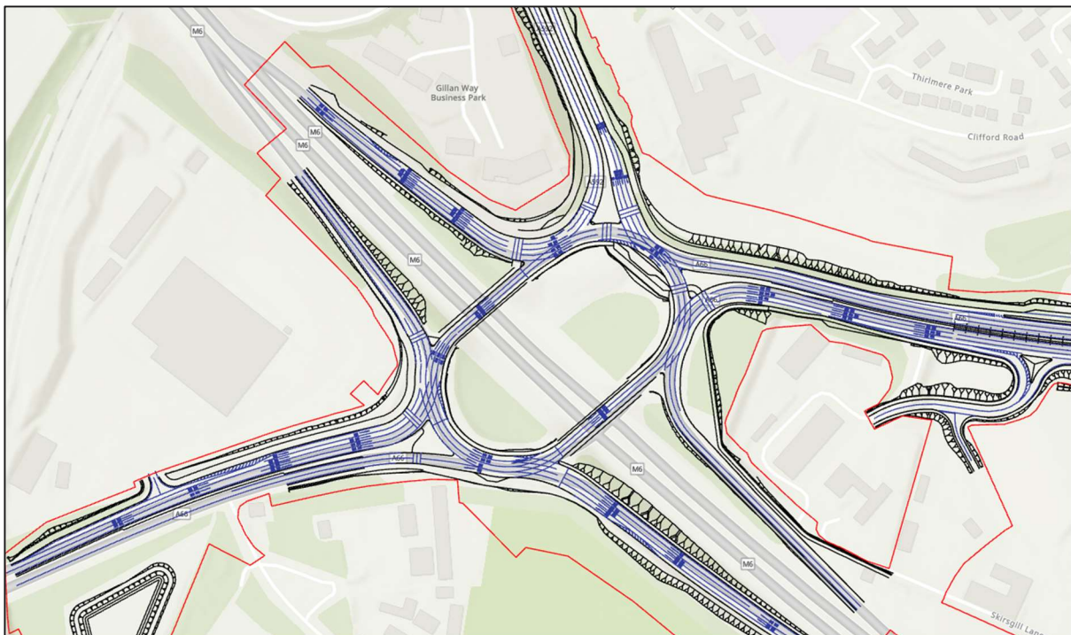
Figure 8-28: M6 J40 scheme design
